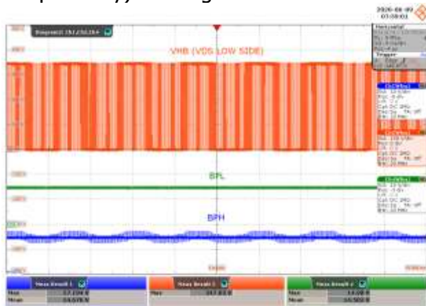
Figure 32 – BPL and BPH Signal at Light Load.
