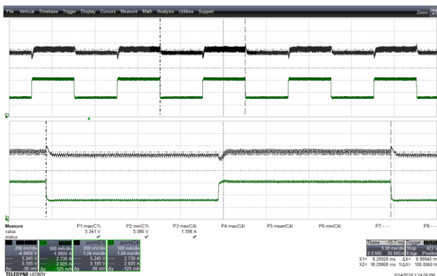
Figure 47 – Transient Response. 85 VAC, 5.0 V, 0.75 – 1.5 A Load Step. V_{MIN} : 5.086 V, V_{MAX} : 5.341 V. Upper: V_{OUT} , 0.2 V / div., 5 ms / div. Lower: I_{LOAD} , 0.5 A / div. Zoom: 1.24 ms / div.
