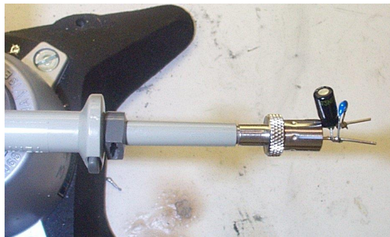
Figure 98 – Oscilloscope Probe with Probe Master ( www.probemaster.com ) 4987A BNC Adapter. (Modified with wires for ripple measurement, and two parallel decoupling capacitors added)
