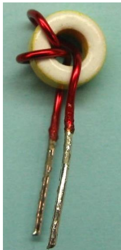
Figure 17 – Finished Part, Front View. Tin Leads to within ~1/8" of Toroid Body.
