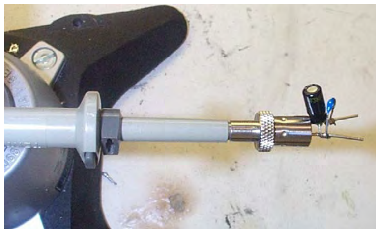
Figure 39 – Oscilloscope Probe with Probe Master ( www.probemaster.com ) 4987A BNC Adapter. (Modified with wires for ripple measurement, and two parallel decoupling capacitors added)
