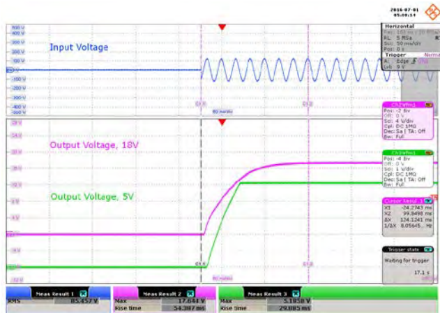
Figure 32 – 85 VAC Input Condition: 18 V – 250 mA, 5 V – 0 A. Upper: V_{IN} , 100 V, 50 ms / div. Middle: V_{OUT1} , 4 V / div. Lower: V_{OUT2} , 1 V / div.
