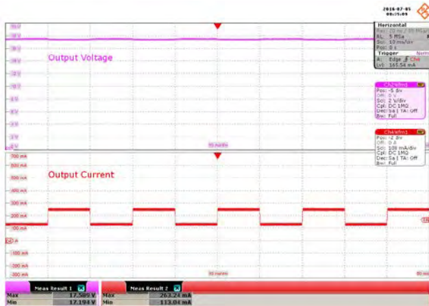
Figure 18 – 85 VAC, 50-100% Load Step. V_{MAX} : 17.589 V. V_{MIN} : 17.194 V. Upper: V_{OUT} , 2 V / div. Lower: I_{LOAD} , 100 mA / div., 10 ms / div.
