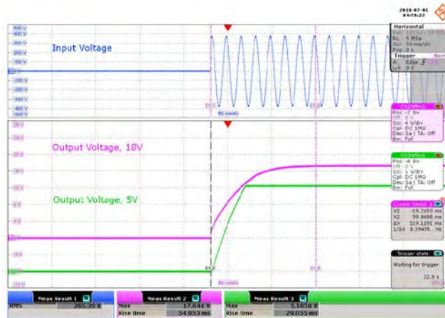
Figure 33 – 265 VAC Input Condition: 18 V – 250 mA, 5 V – 0 A. Upper: V_{IN} , 100 V, 50 ms / div. Middle: V_{OUT1} , 4 V / div. Lower: V_{OUT2} , 1 V / div.
