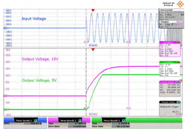
Figure 35 – 265 VAC Input. Condition: 18 V – 250 mA, 5 V – 50 mA. Upper: V_{IN} , 100 V, 50 ms / div. Middle: V_{OUT1} , 4 V / div. Lower: V_{OUT2} , 1 V / div.
