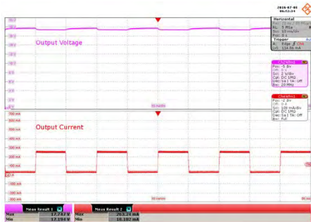
Figure 20 – 85 VAC, 10-100% Load Step. V_{MAX} : 17.747 V. V_{MIN} : 17.194 V. Upper: V_{OUT} , 2 V / div. Lower: I_{LOAD} , 100 mA / div., 10 ms / div.
