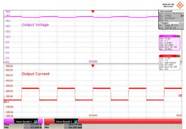
Figure 21 – 265 VAC, 10-100% Load Step. V_{MAX} : 17.747 V. V_{MIN} : 17.194 V. Upper: V_{OUT} , 2 V / div. Lower: I_{LOAD} , 100 mA / div., 10 ms / div.
