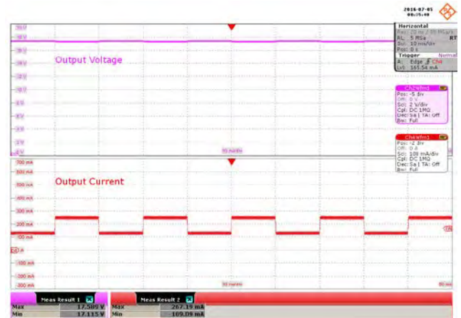
Figure 19 – 265 VAC, 50-100% Load Step. V_{MAX} : 17.589 V. V_{MIN} : 17.115 V. Upper: V_{OUT} , 2 V / div. Lower: I_{LOAD} , 100 mA / div., 10 ms / div.
