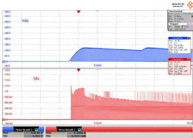
Figure 28 – 85 VAC Input. Condition: 18 V – 250 mA, 5 V – 50 mA. Upper: V_{DRAIN} , 50 V, 5 ms / div. Lower: I_{DRAIN} , 200 mA / div.
