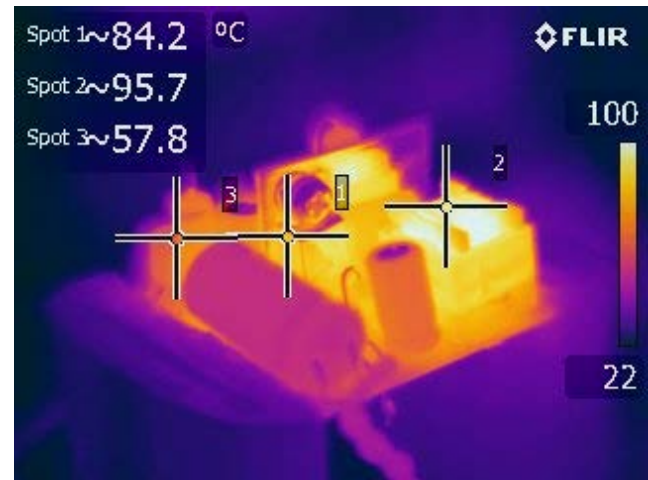
Figure 22 – 230 VAC, Full Load. Spot 1: LYT4326E. Spot 2: Transformer. Spot 3: Damping Resistor.
