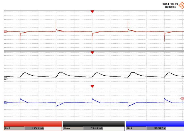
Figure 60 – 49° Conduction Angle. Upper: I_{IN} , 500 mA / div. Middle: I_{OUT} , 50 mA / div. Lower: V_{IN} , 200 V / div., 5 ms / div.
