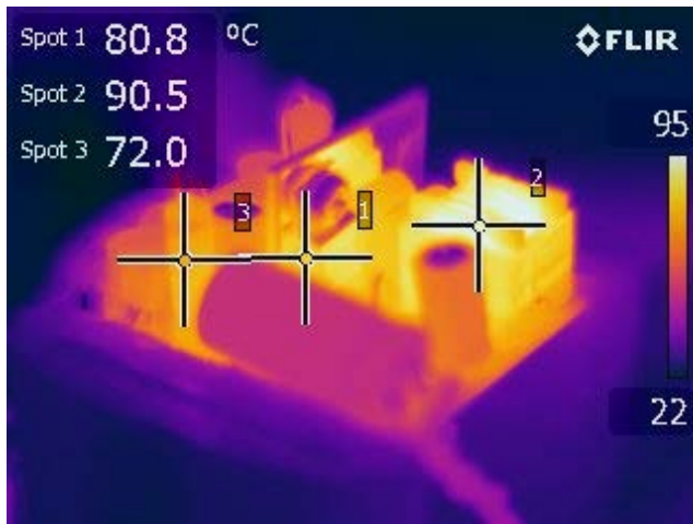
Figure 21 – 195 VAC, Full Load. Spot 1: LYT4326E. Spot 2: Transformer. Spot 3: Damping Resistor.
