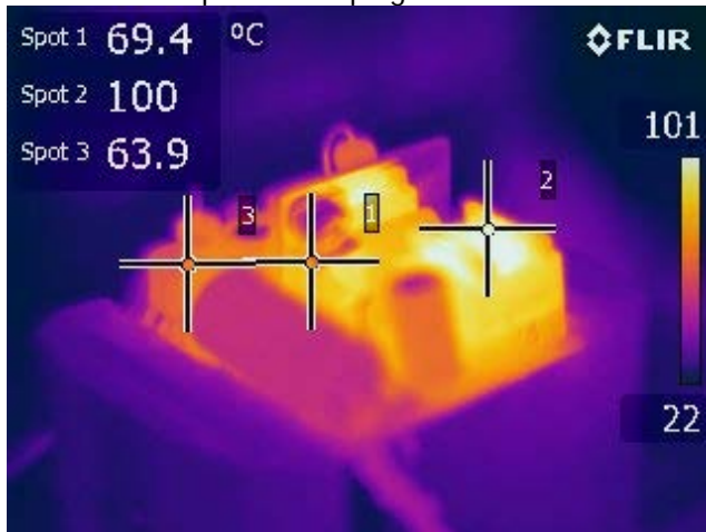
Figure 23 – 265 VAC, Full Load. Spot 1: LYT4326E. Spot 2: Transformer. Spot 3: Damping Resistor.
