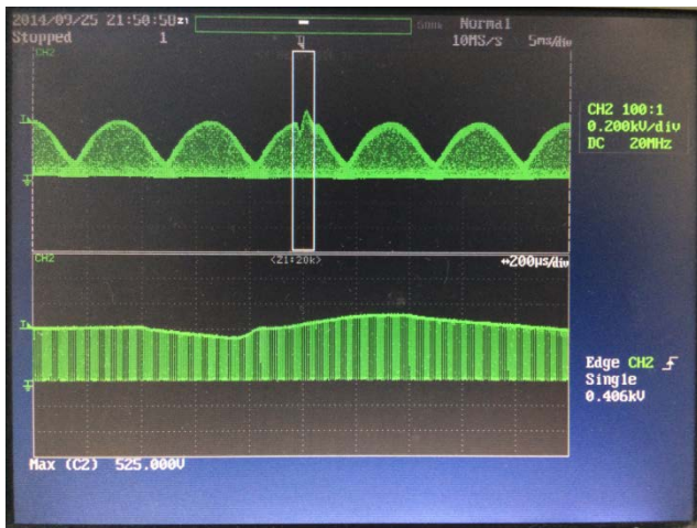
Figure 66 – 230 VAC, +2.5 kV Ring Wave, 90° V_{DRAIN} , 200 V / div., 5 ms / div.
