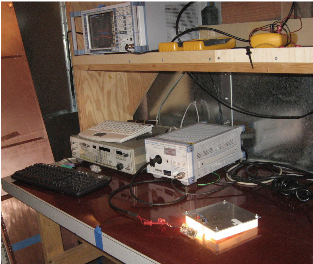
Figure 48 – Conducted Emissions Measurement Set-up.
