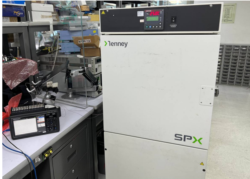
Figure 48 – Thermal Chamber Test Set-up.
