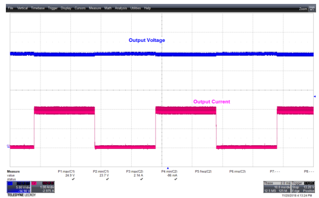
Figure 41 – 265 VAC 50 Hz, 0 A – 1.88 A Transient Load. Upper: V_{OUT} , 5 V / div. Lower: I_{OUT} , 1 A / div., 10 ms / div.
