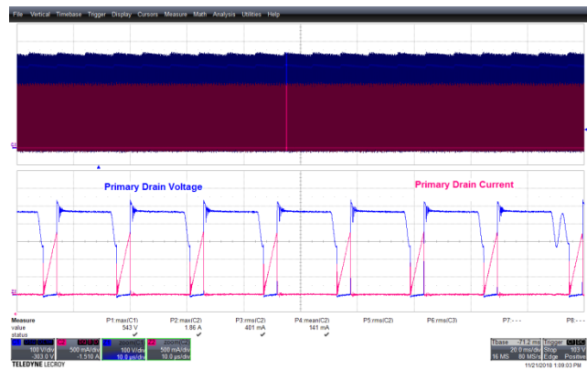
Figure 61 – 265 VAC 60 Hz, 15 V Full Load Normal. Upper: I_{DRAIN} , 500 mA / div. Lower: V_{DRAIN} , 100 V / div., 10 \mu\text{s} / div. I_{DS} = 1.86\text{ A} , V_{DS} = 543\text{ V} .
