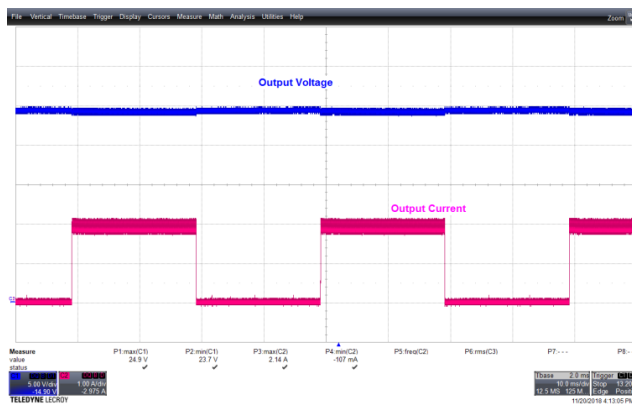
Figure 40 – 230 VAC 50 Hz, 0 A – 1.88 A Transient Load. Upper: V_{OUT} , 5 V / div. Lower: I_{OUT} , 1 A / div., 10 ms / div.
