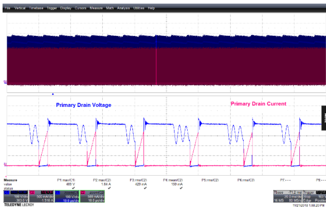
Figure 60 – 230 VAC 60 Hz, 15 V Full Load Normal. Upper: I_{DRAIN} , 500 mA / div. Lower: V_{DRAIN} , 100 V / div., 10 \mu\text{s} / div. I_{DS} = 1.84\text{ A} , V_{DS} = 489\text{ V} .
