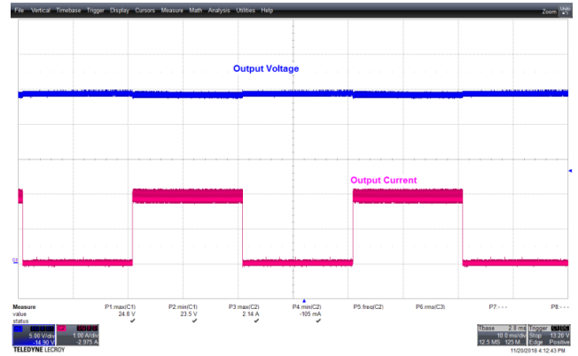
Figure 39 – 115 VAC 60 Hz, 0 A – 1.88 A Transient Load. Upper: V_{OUT} , 5 V / div. Lower: I_{OUT} , 1 A / div., 10 ms / div.
