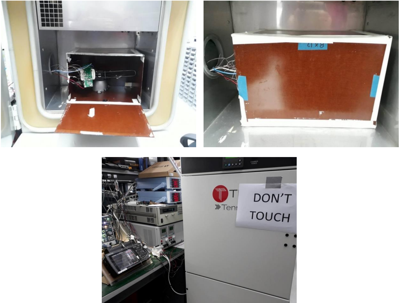
Figure 48 – Test Set-up Picture Thermal at 50 °C Ambient - Open Frame.
