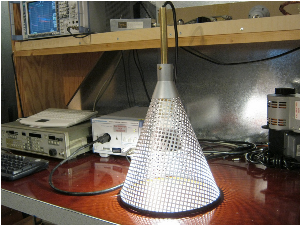
Figure 48 – EMI Test Set-up with the Unit and LED Load Placed Inside the Cone.
