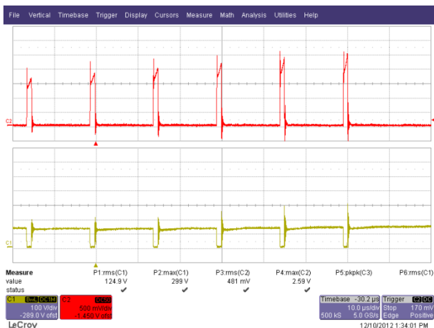
Figure 54 – 132 VAC, 60 Hz Start-up. Upper: I_{DRAIN} , 500 mA / div. Lower: V_{DRAIN} , 100 V, 10 \mu s / div.
