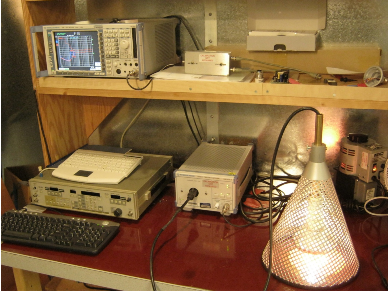
Figure 63 – EMI Test Set-up with the Unit and LED Load Placed Inside a Conical Metal Housing as Described in CISPR 15 / IEC: 2005 Standard.
