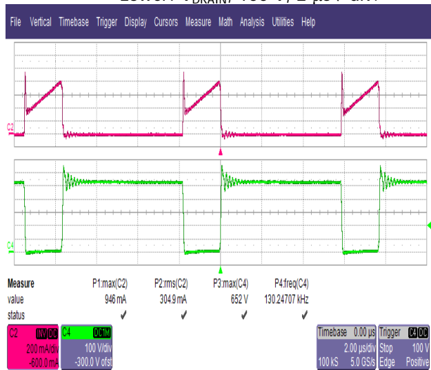
Figure 23 – 400 VDC, Over Load (125%). Upper: I_{DRAIN} , 0.2 A / div. Lower: V_{DRAIN} , 100 V, 2 \mu s / div.
