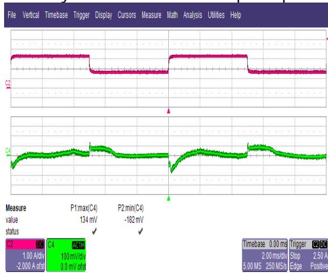
Figure 31 – Transient Response, 380 VDC. 50-100-50% Load Step. Upper: I_{LOAD} , 1 A / div. Lower: V_{OUT} , 0.1 V / div., 2 ms / div.
