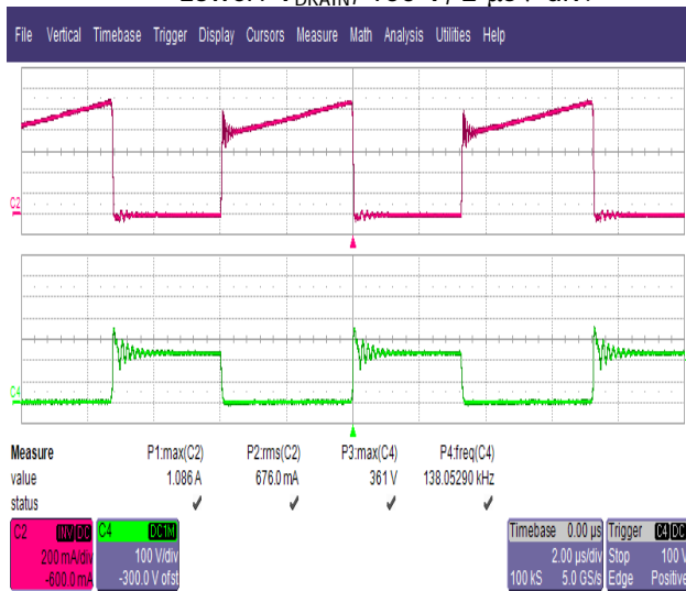
Figure 22 – 110 VDC, Over Load (125%). Upper: I_{DRAIN} , 0.2 A / div. Lower: V_{DRAIN} , 100 V, 2 \mu s / div.
