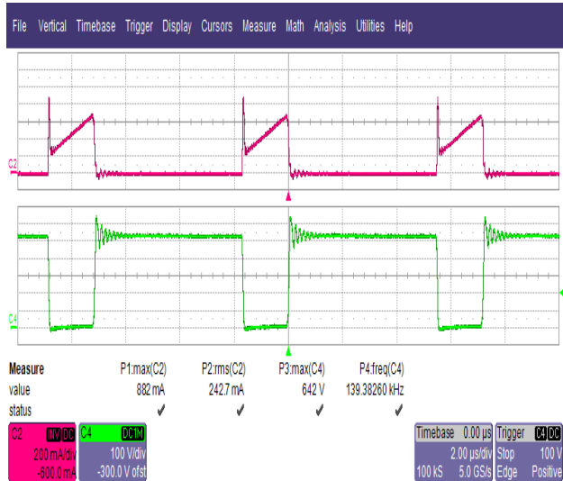
Figure 21 – 400 VDC, Full Load. Upper: I_{DRAIN} , 0.2 A / div. Lower: V_{DRAIN} , 100 V, 2 \mu s / div.
