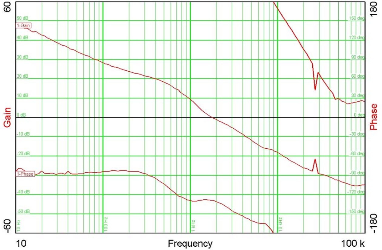
Figure 36 – Gain-Phase Plot, Maximum Steady-State Load. Vertical Scale: Gain = 10 dB / div., Phase = 30 ° / div. 110 VDC – Crossover Frequency = 1.8 kHz Phase Margin = 50°.
