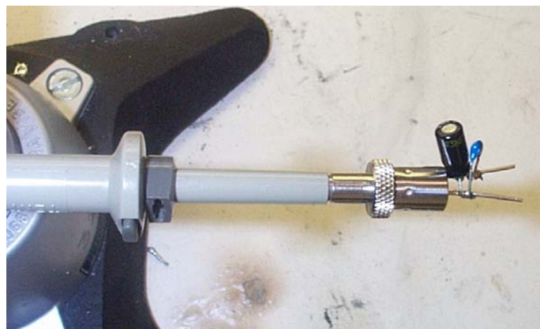
Figure 32 – Oscilloscope Probe with Probe Master ( www.probemaster.com ) 4987A BNC Adapter. (Modified with wires for ripple measurement, and two parallel decoupling capacitors added)
