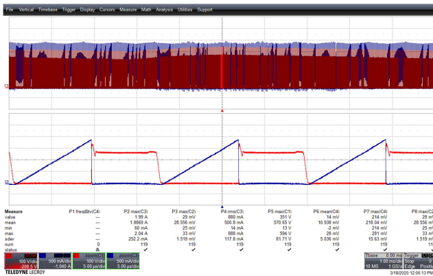
Figure 27 – Drain Voltage and Current Waveforms. 90 VAC, 100% Load. C1/Z1 : V_{DRAIN} , 100 V / div. C3/Z3 : I_{DRAIN} , 0.5 A / div., 5 \mu s / div.
