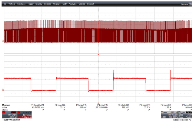
Figure 29 – SR FET Voltage Waveforms. 90 VAC, 100% Load, (37.0 V MAX ). C1: SR_V DRAIN , 10 V / div., 5 μs / div.
