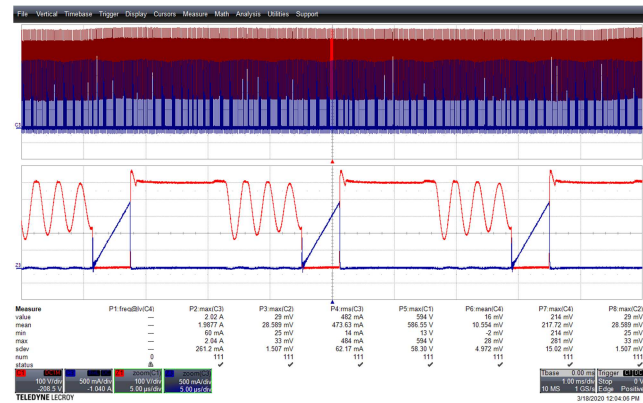
Figure 28 – Drain Voltage and Current Waveforms. 265 VAC, 100% Load. C1/Z1 : V_{DRAIN} , 100 V / div. C3/Z3 : I_{DRAIN} , 0.5 A / div., 5 \mu s / div.
