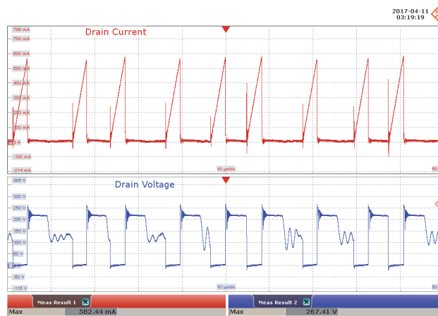
Figure 66 – 90 VAC 60 Hz, Full Load Normal. Upper: I_{DRAIN} , 100 mA / div. Lower: V_{DRAIN} , 50 V / div., 10 \mu s / div.
