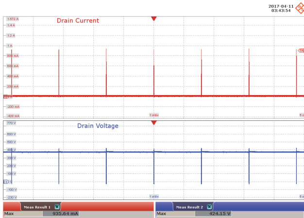
Figure 79 – 265 VAC, Output Shorted. Upper: I_{DRAIN} , 200 mA / div. Lower: V_{DRAIN} , 100 V / div., 1 s / div.
