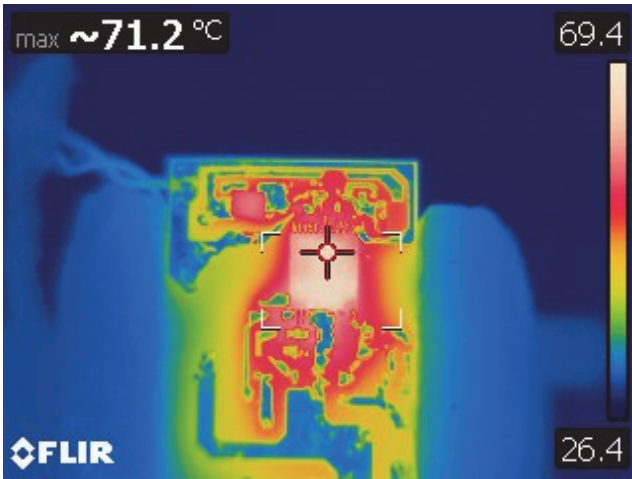
Figure 32 – 230 VAC 50 Hz, Full Load. LYTSwitch-6 (U1): 71.2 °C.
