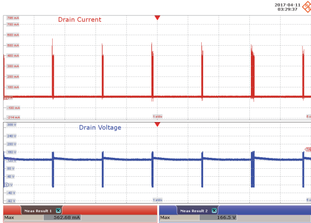
Figure 77 – 90 VAC 60 Hz, Output Shorted. Upper: I_{DRAIN} , 100 mA / div. Lower: V_{DRAIN} , 40 V / div., 1 s / div.
