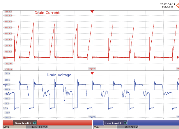
Figure 68 – 115 VAC 60 Hz, Full Load Normal. Upper: I_{DRAIN} , 100 mA / div. Lower: V_{DRAIN} , 50 V / div., 10 \mu s / div.
