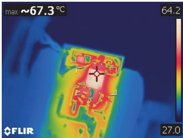
Figure 28 – 115 VAC 60 Hz, Full Load. LYTSwitch-6 (U1): 67.3 °C.
