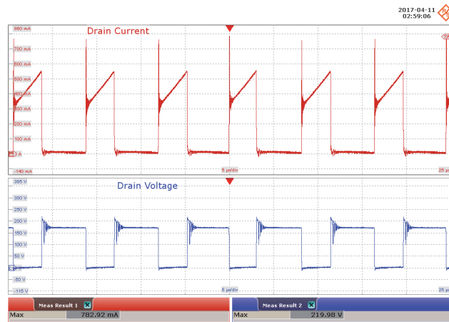
Figure 74 – 90 VAC 60 Hz, Full Load Start-up. Upper: I_{DRAIN} , 100 mA / div. Lower: V_{DRAIN} , 50 V / div., 5 \mu s / div.
