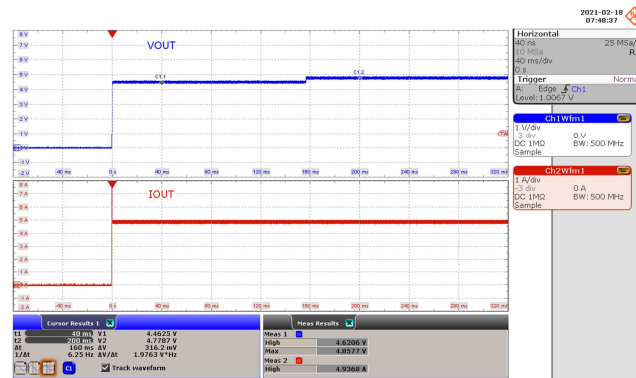
Figure 56 – Output Voltage and Current. 265 VAC, 5.0 V, 5 A (CC Mode). V_{OUT} = 4.7787 V Steady-State. CH1: V_{OUT} , 1 V / div. CH2: I_{LOAD} , 1 A / div. Time: 40 ms / div.
